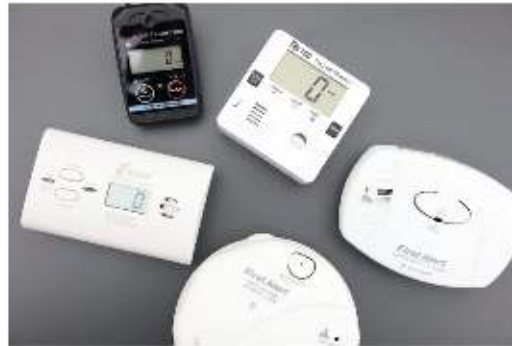
An array of portable carbon monoxide monitors, which range in cost from $20 to $200 and have different levels of sensitivity. — Kristina Barker for The New York Times
